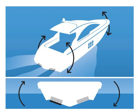
IS provides perfect control of pitch and heel. In Auto mode, IS constantly optimizes the boat's attitude in all directions.
